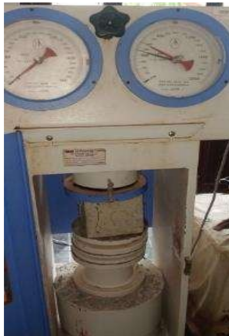
Fig :2 Cube under compression testing machine
