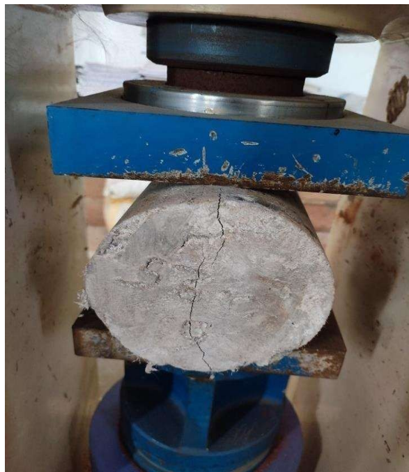
Fig:3 Cylinder under compression testing machine
